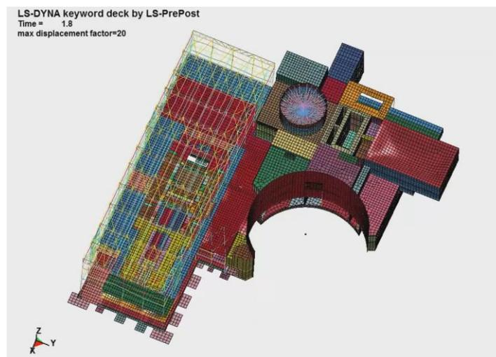
Fig. 2. LS-DYNA seismic analysis of nuclear power plant buildings
