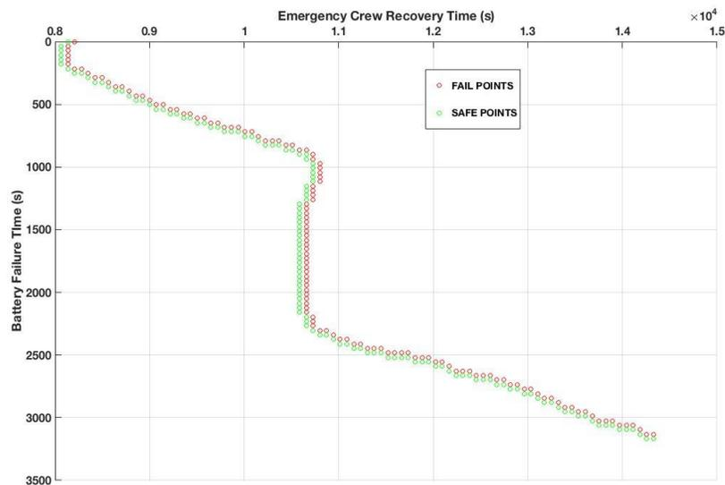
Fig. 5. RELAP5-3D/RAVEN limit surface for SBO scenario.
