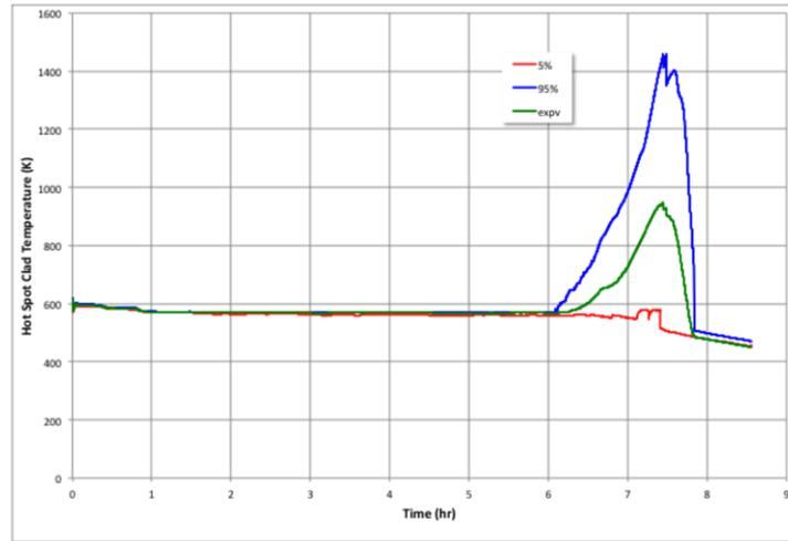
Fig. 4. Uncertainty bands for BEPU RELAP5-3D/RAVEN calculation for a LOOP scenario.
