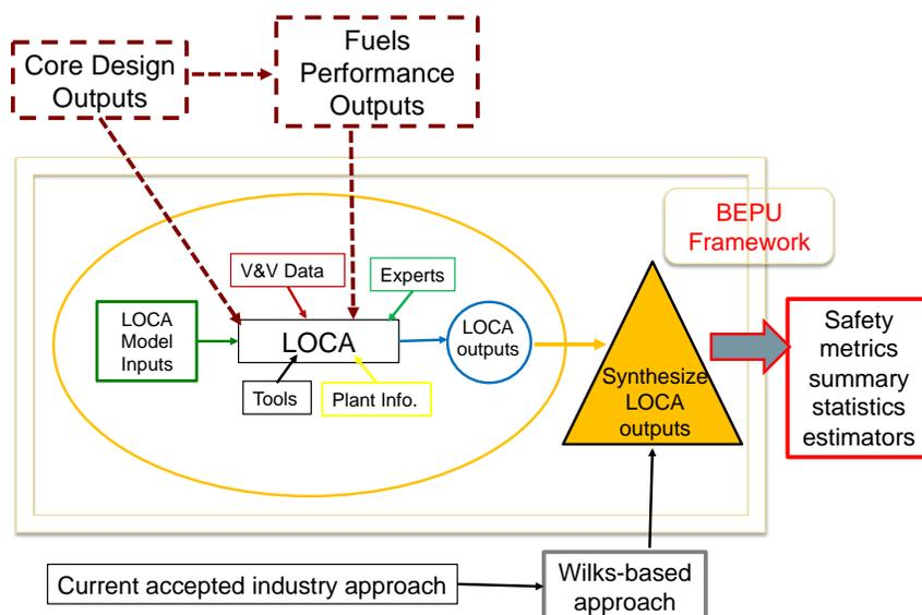
Figure 1. Schematic illustration of the current BEPU process for LOCA analysis
