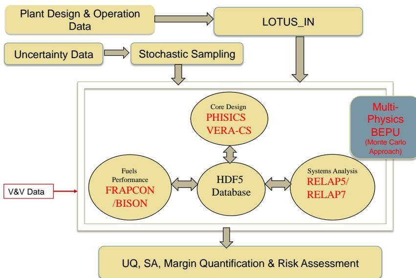
**Figure 3. Illustration of LOTUS Multi-Physics BEPU (MP-BEPU) safety analysis framework.**
