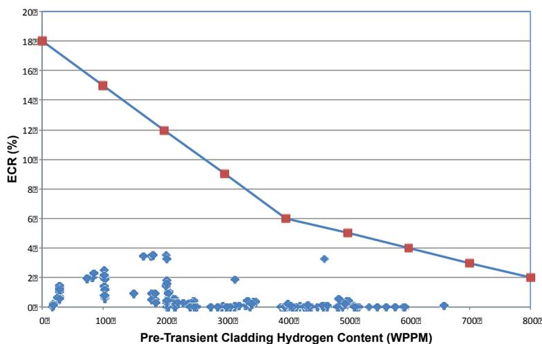
**Figure 4. RELAP5-3D calculated ECR vs. acceptance criterion in NRC proposed new rulemaking in 10 CFR 50.46c.**
